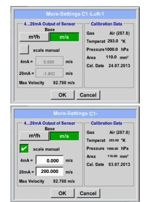
In *More-Settings*, you can define whether the 4 - 20 mA analogue output of the sensor based on the flow rate or velocity.
