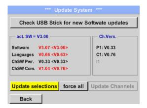
If the PI 500 is correctly connected to USB, and new version available it will displayed.
