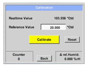
Here, a one-point calibration can be performed.
