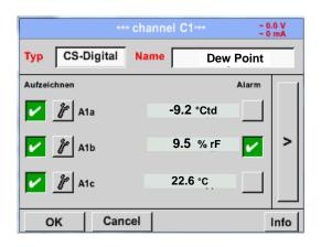
The PI 500 detects, if the connected sensor is a flow or dew point sensor of **CS Instruments** and set the CS-Digital subtype automatically correct.
