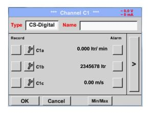
The PI 500 detects, if the connected sensor is a flow or dew point sensor of **CS Instruments** and set the CS-Digital subtype automatically correct.
