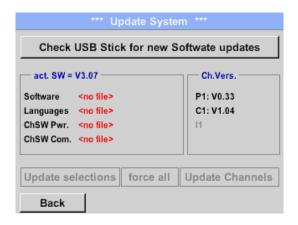
If after pushing the *Check USB Stick for new Software updates* button the following messages in the window appears, then PI 500 is not connected properly with the USB stick or no files are available.
