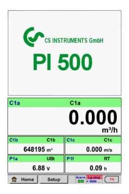
After switching on the PI 500 the channel is initialized and the menu " *Real time values* " appears.
