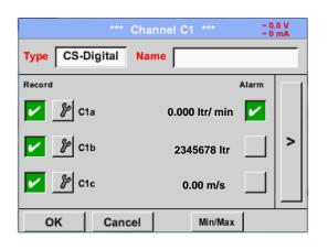
After alarm setting for Channel C1a.
