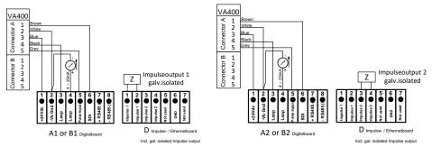
For systems with 2 digital boards (2x2 digital channels) on pulse output 1 could be used either pulse input A1 or B1, as well as for pulse output 2 either pulse input A2 or B2.
