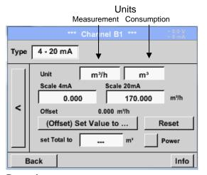
Selection of the units by pushing the text fields for the corresponding measurement and consumption units. In addition, you can push the *scale buttons* for the min. and max. scaling values and set the measuring range. Here we have  $0 \text{ m}^3/h$  for 4 mA and 170m<sup>3</sup>/h for 20mA In addition it is possible to enter a starting value for consumption entering *set Total to* field e.g. to take over value from an old counter. Confirmation of the inputs by pushing button *OK*
