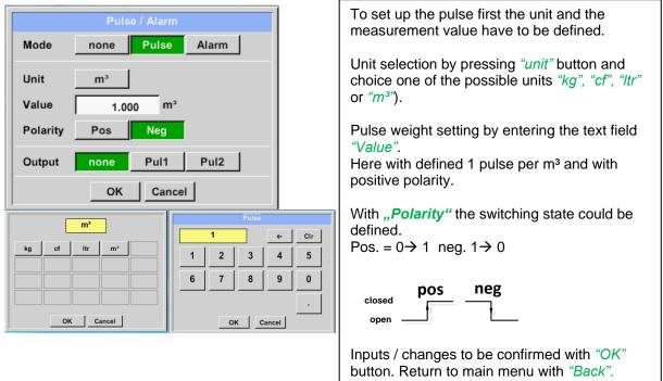
Furthermore, the DS400 also offers the option to provide the pulses, galvanically isolated, directly, this requires the option boards "Pulse" or "Ethernet"
