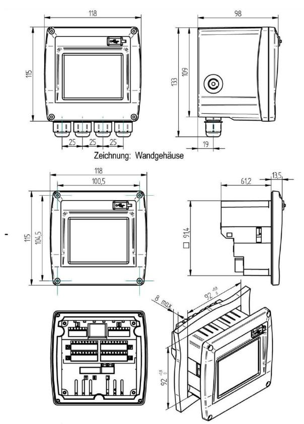
Figure : Housing for panel mounting
