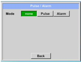
The pulse output of the VA 5xx could be set functionally as pulse output or alarm output.
