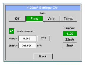
This menu allows the adjustment / assignment of the measurement value and the scaling of the analogue output by pressing the "4-20mA Ch1" button.
