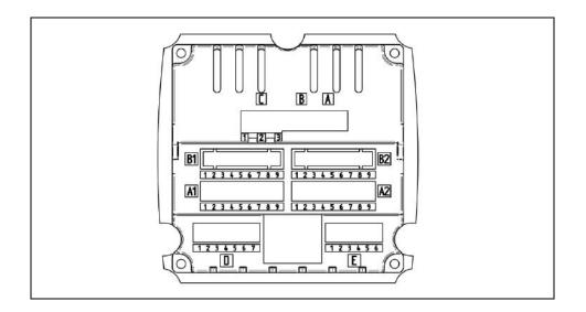
10.1 Connections Inputs "A1 – B2" (Analog- und Digital-Channels)
