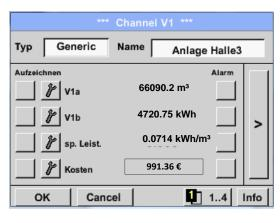
Result in *V1b* is the energy consumption read out from the energy counter.
