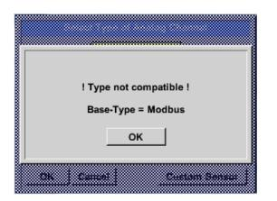
In case a wrong (not compatible) Sensor type (analogue / digital) has selected an error message will be displayed.
