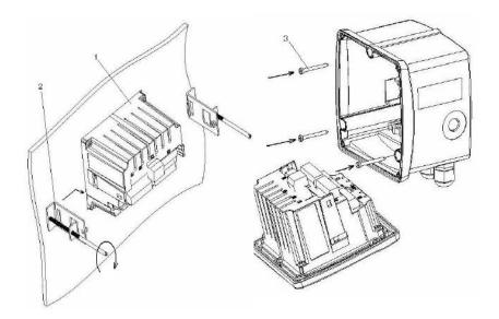
Figure: Panel and wall mountable housing
