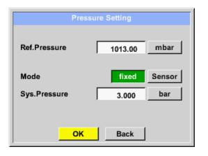
The definition of the fixed value system pressure value is done by activating the button "fixed", but this is only required in case a ext. pressure probe is connected. The value is entered in the corresponding text
