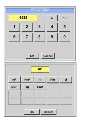
The sensor allows taking over a starting counter value. Inserting the value by entering the "*Count. Val.*" text field.
