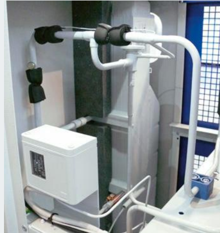
Inside of coated refrigeration dryer
